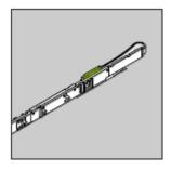
**End of run** is terminated by folding the last flag back and connecting it to its own powerblock terminal.
